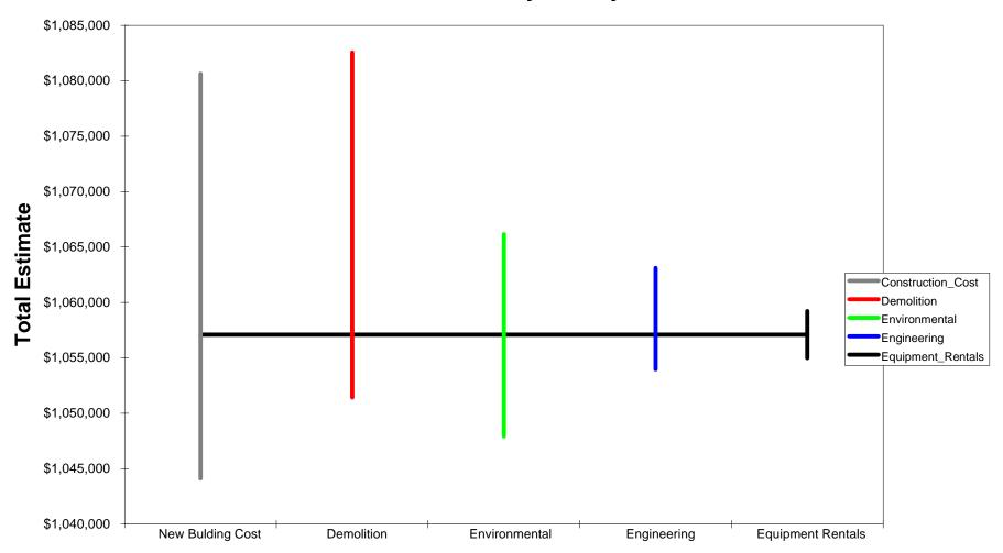
The horizontal line represents the study case. A vertical line represents the output variable range between an input variable's 10% likely and 90% likely values. Input variables with long vertical lines have the most effect on the output variable.
