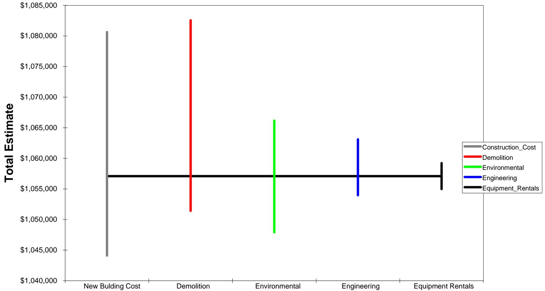
The horizontal line represents the study case. A vertical line represents the output variable range between an input variable's 10% likely and 90% likely values. Input variables with long vertical lines have the most effect on the output variable.
